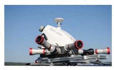
The RIEGL VMX-2HA is a high speed, high performance dual scanner Mobile Mapping System which provides dense, accurate, and feature-rich data at highway speeds. The VMX line of systems has been RIEGL's flagship mobile mapping system for 14 years.
