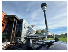
The RIEGL VMY-1 is an economically priced Mapping System of small dimensions, that is well suited for a variety of mobile mapping applications. The VMY-1 is also set up for the sensor to be quickly converted to an integration for a variety of drone platforms.
